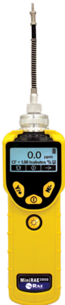
FIGURE 2.5.2. MiniRAE 3000 portable PID
